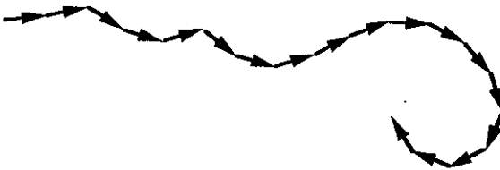
Figure 1. A representation of a dipoled chain. The chain can bend but it cannot stretch. It is thus worm-like. Non-dipolar spacers may be put in between the dipoles to allow more flexibility.
